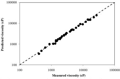
Figure 2. Comparison between measured and predicted viscosity values
