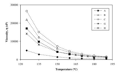
Figure 1. Temperature-viscosity curves of the asphalt rubber binders
