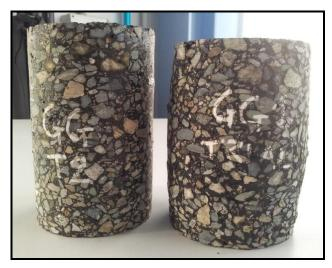
Figure 2 – AMPT specimens after FN testing
